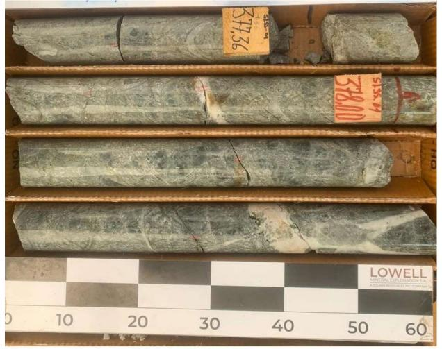
Notes to Figure 4: SLSS-01 core interval from 377.03 to 379.15m, averaging 0.74% Cu, 0.04% Mo and 0.05g/t Au. Quartz-diorite intermineral dike is cutting andestic volcanics. Alteration and mineralization is mainly composed of early-stage, halo-type associations with quartz, anhydrite, chlorite, biotite, epidote, pyrite, chalcopyrite, and magnetite cut by A- and B-type Mo-bearing quartz veinlets.
