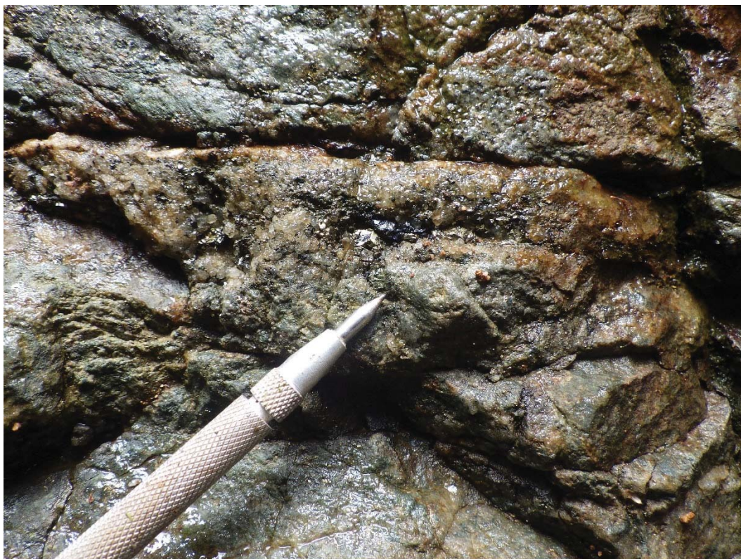
Figure 12.2. Closeup of sericite-altered porphyry cut by pyrite-chalcocite veins consistent with the supergene enriched zone of the deposit. Photo taken from a large outcrop exposure within a creek about 80 m west of drill site W12 within Warintza Central.
